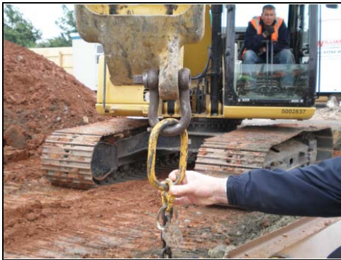
Figure 1 - Master link rotation restricted to approx \pm 70^\circ
