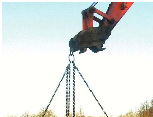
Figure 5 – Chain and master link can hang freely without obstruction
